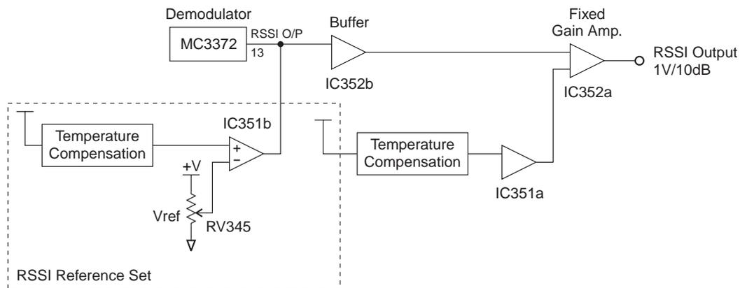
**Figure 2.7 T885 RSSI Block Diagram**
