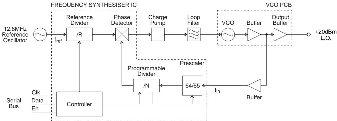
**Figure 2.6 T885 Synthesiser Block Diagram**
