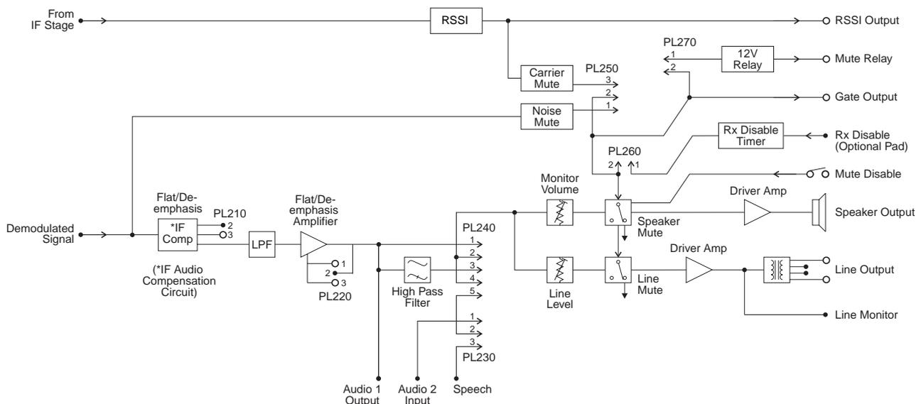
Figure 2.3 T885 Audio Processor Block Diagram
